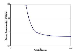
Figure 2. Plot showing the increase in energy consumption as toner particle size is reduced.
