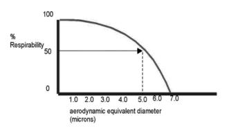
Figure 4. British Medical Research Council penetration curve for respirable particles showing 50% cut point at 5 µm.
